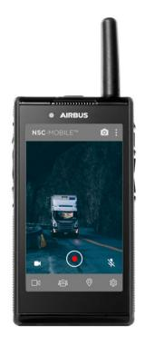
**NSC Mobile** is the personal level sensor data source client, designed to be used in devices such as mobile phones, wearable cameras and other hand held devices and accessories. Secure PTT and Chat service with team tracking.
